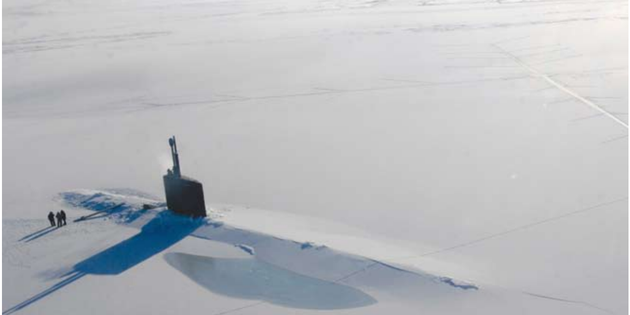
The Los Angeles-class submarine USS Annapolis (SSN 760) broke through three feet of ice during Ice Exercise (ICEX) 2009 in the Arctic Ocean. ICEX 2009 was intended to test and evaluate naval submarine operability in the changing Arctic environment. (MASS COMMUNICATION SPECIALIST 1ST CLASS TIFFINI M. JONES/U.S. Navy)
